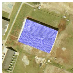
Figure 3: Interpolated LIDAR points on the roof
