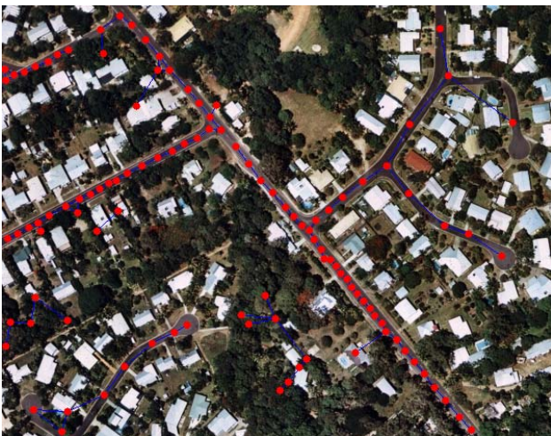
Figure 3. Growing Neural Gas has produced this road network based on simple image operations
