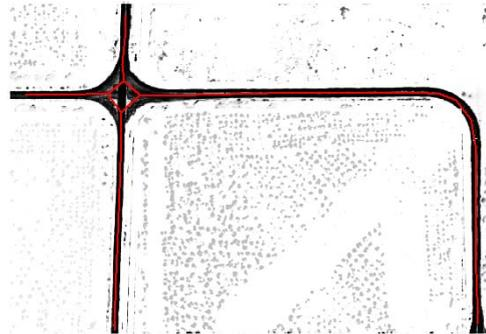
Figure 12. Road vectorization of input image 7a
