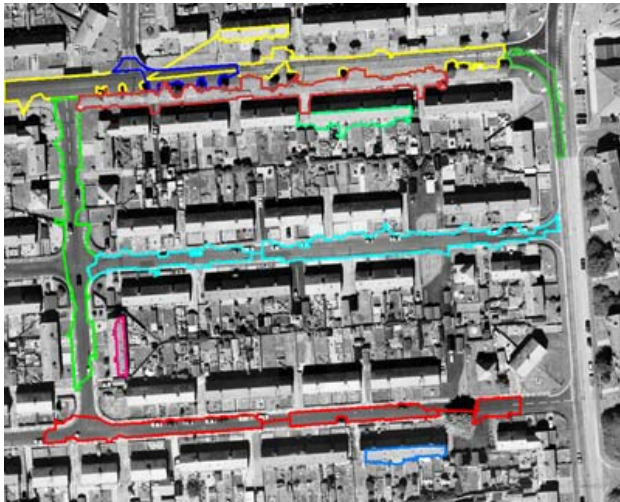
Figure 6. Assembled road parts. Connections between road parts are shown as lines in the same colour. Intensity image used for clarity of display.
