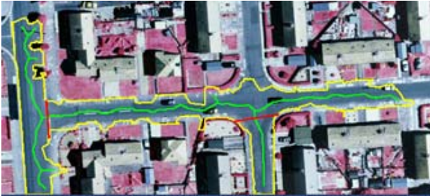
Figure 1. Partition of large segment. Original segment borders in yellow, skeleton in green, dividing lines in red.
