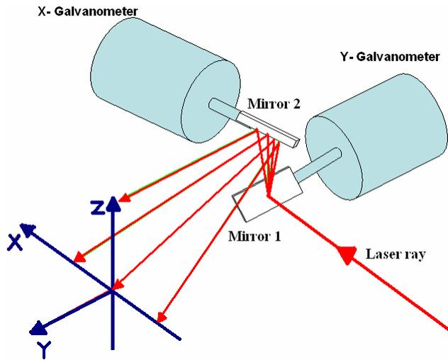
Figure 3. XY-Scanner
