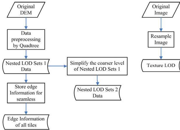
Figure 1. Procedure of data pre-processing.
