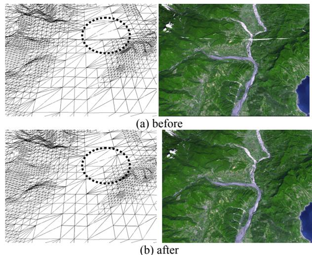
Figure 11. Visual effect of T-junctions removal.
