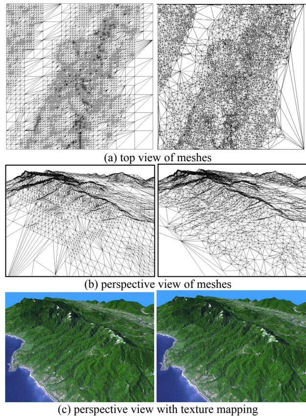
Figure 8. Comparison between Quadtree (left) and Delaunay (right) LODs.
