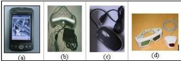
Figure 2. (a) A typical PDA ;( b) the 3D mouse; (c) regular mouse with trolley; (d) stereo glasses and radiator
