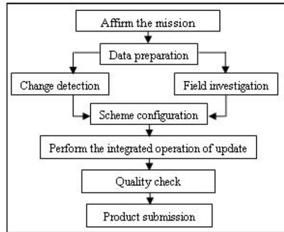
Figure 1. The update workflow with the operation mode of integration
