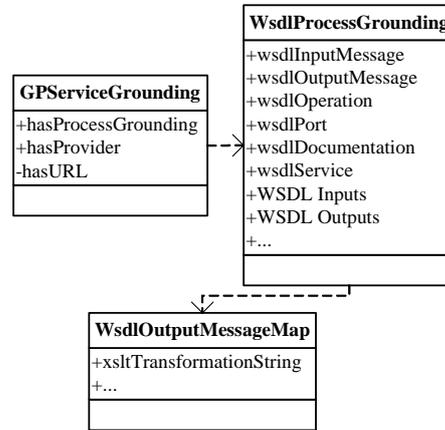
Figure 6. GPServiceGrounding Ontology
