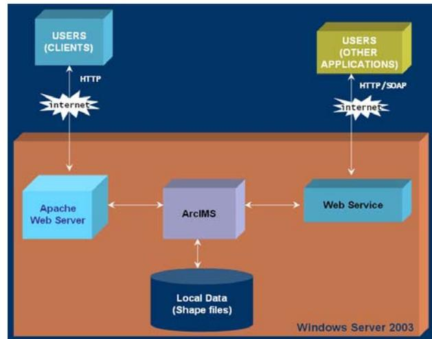
Figure 2. System architecture
