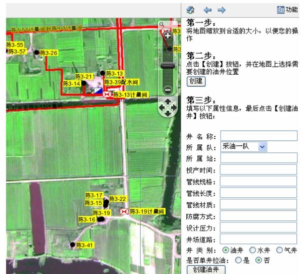
Figure 6. The guideline telling how to create a new oil well information
