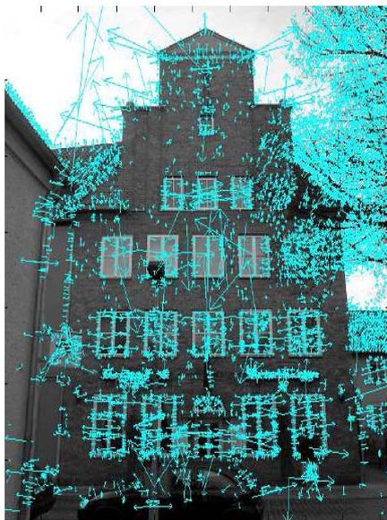
Figure 4. SIFT features extracted in reference image
