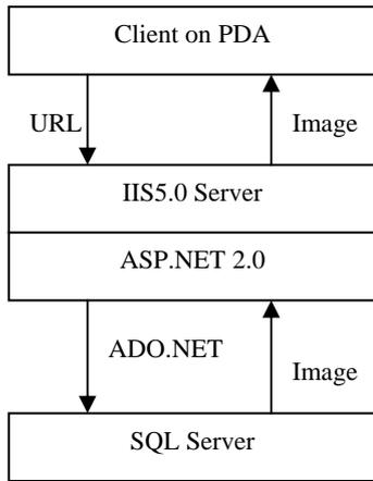
Figure 4. Structure of the prototype system
