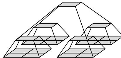
Figure 3. Structure of an image pyramid
