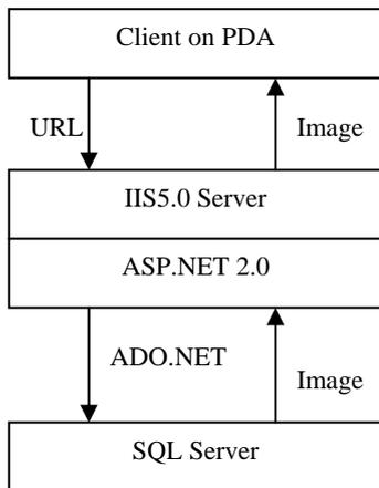
Figure 4. Structure of the prototype system
