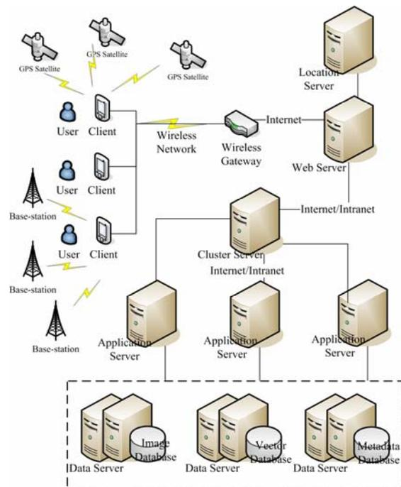
Figure 2. Architecture of remote sensing mobile service
