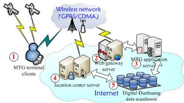
Figure 3: MTG architecture and application workflow
