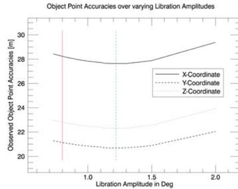
Figure 6: Observed residuals of object points for varying forced libration amplitudes. The red vertical line indicates the observation by (Duxbury, 1991), the green line indicates the minimum of SRC observations.
