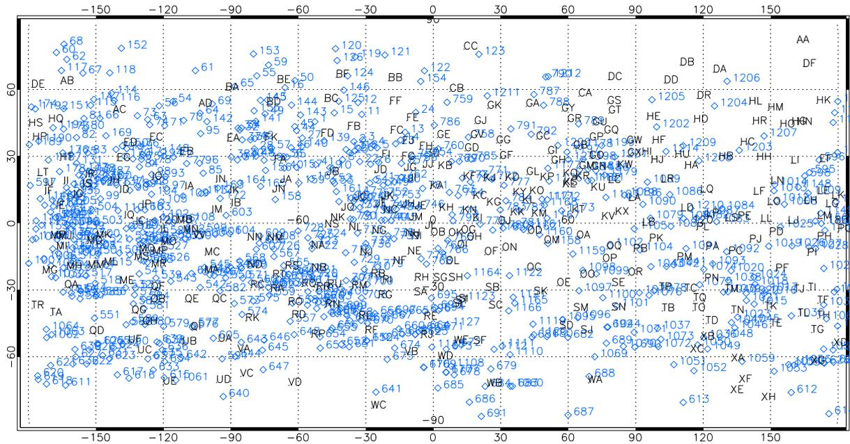
Figure 4: Control points (blue) of the DLR network in comparison with the Duxbury and Callahan control point network (letters). The density has increased by a factor of two while the uncertainty of the control point coordinates is approx. a 6 times lower.
