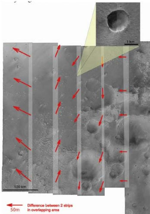
Figure 4. Results of single strip adjustment (planimetry)
