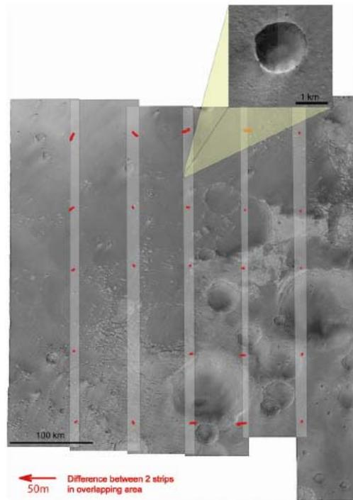
Figure 6. Results of bundle block adjustment (planimetry)
