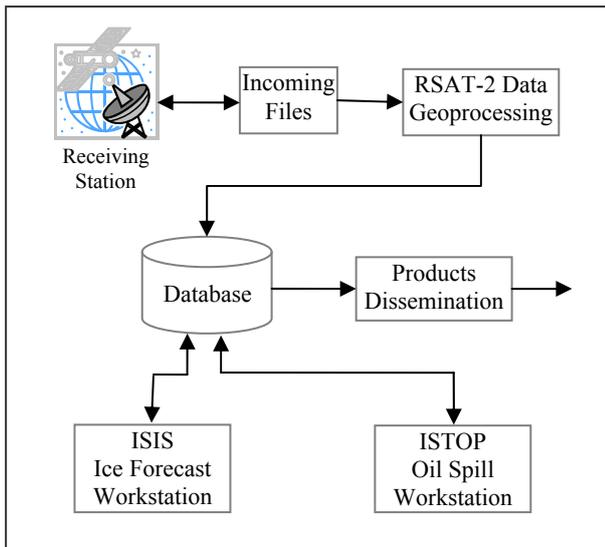
Figure 6: Data Processing Flow Diagram
