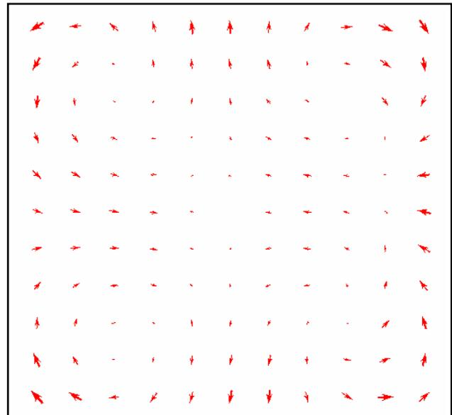
Figure 5: Total Errors for a 2nd Order Global Polynomial Transformation (RMS: 0.96 Pixel)
