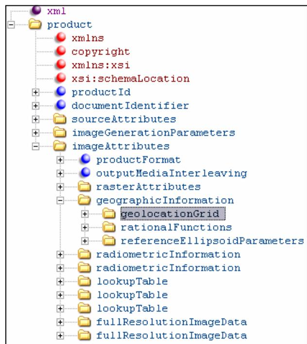
Figure 2: RADARSAT-2 Product XML Node Tree
