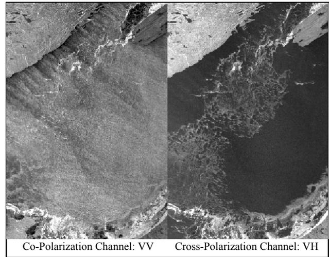
Figure 7: Co-Polarization vs Cross-Polarization at High Wind Condition
