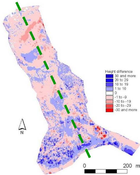
Figure 8 Difference of DSM between the years 2006 and 2007.
