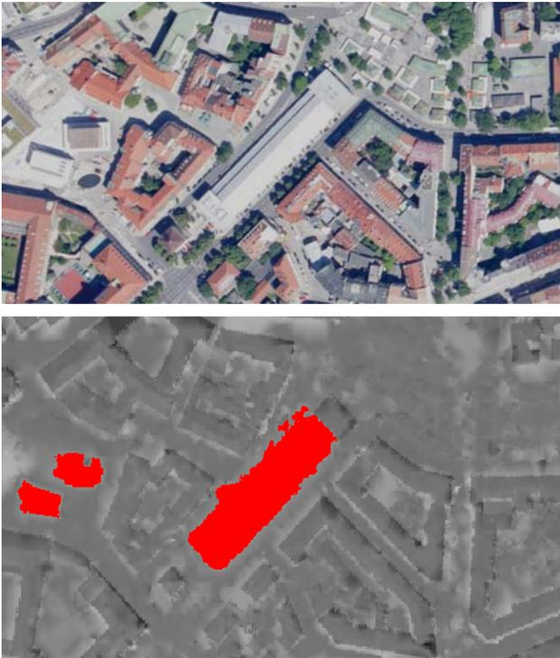
Figure 11 Difference between the 3K DSM from 17<sup>th</sup> June 2007 and the LIDAR DEM (bottom) and the corresponding orthophoto (top).
