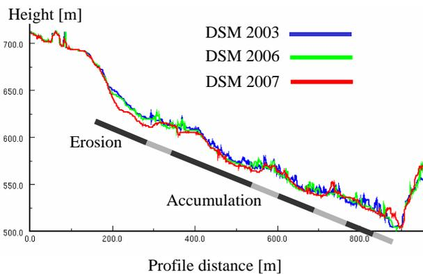
Figure 9 Profile through DSMs of the years 2003, 2006, and 2007.
