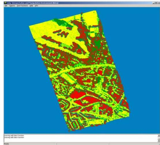
Figure 2 Bournemouth (2005) DSM collected by the NGATE Socet Set extraction module after classification with TerraScan.
