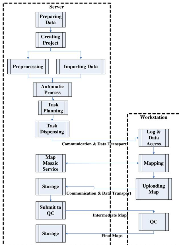
Figure 7. Workflows of seamless mapping system
