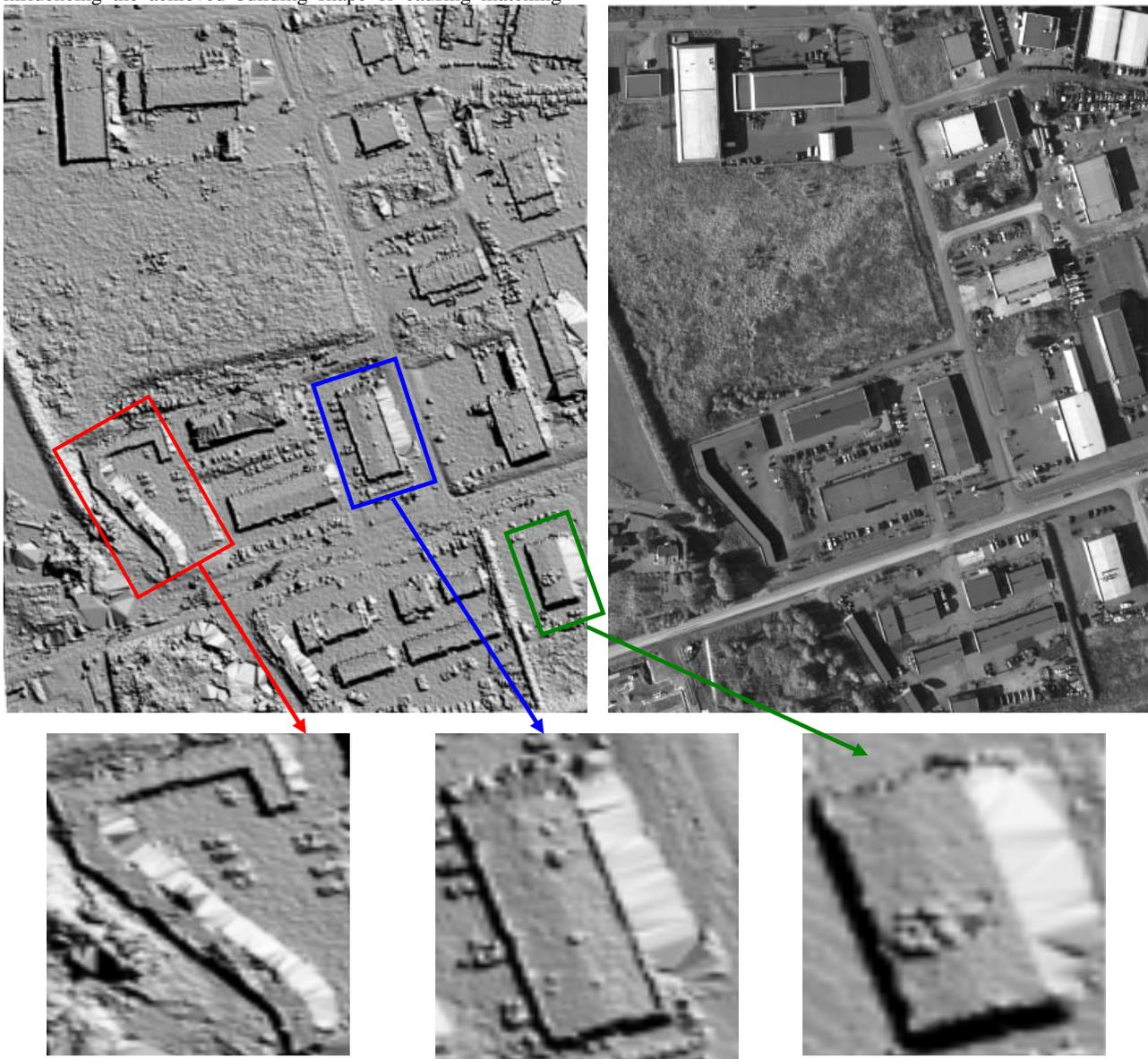
Figure 7: Shaded visualization of matched DSM with some details, upper right = DMC-image
