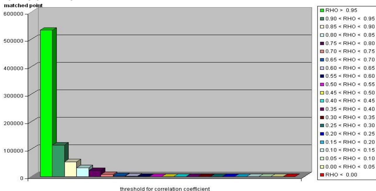
Optimal results have been achieved in the area with man-made objects with the threshold for the correlation coefficient  $R=0.70$  of the least squares matching, the sub-matrix of  $10 \times 10$  pixels and the step width of 3 pixels. A lower threshold for the correlation coefficient may lead to a lower accuracy, requiring a compromise between both.
