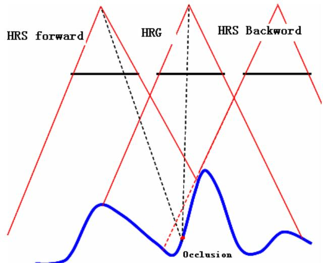
Figure 5. Combination of HRG and HRS images for stereoscopic measurements of DLG
