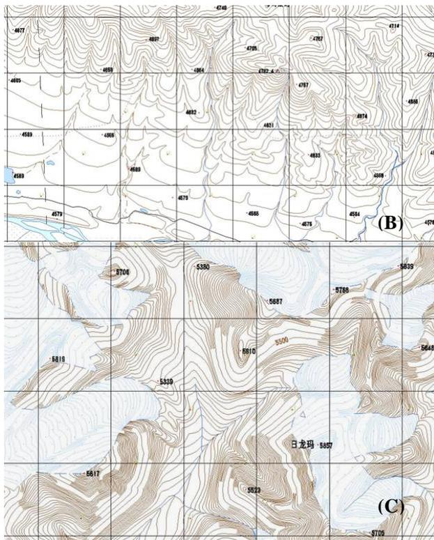
Figure 6. DLGs collected by stereoscopic measurements from SPOT-5 HRS and HRG image stereo pairs. (A) is a DLG of an alluvial flat area. (B) is a DLG of a hilly terrain area. (C) is a DLG of a glacial landform area.
