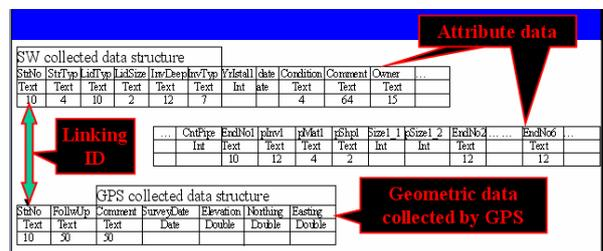
Figure 2. The SW Field Data Organization/Linking with GPS Data
