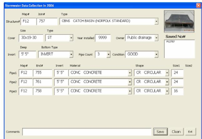
Figure 4. Storm Water Field Data Entry Form
