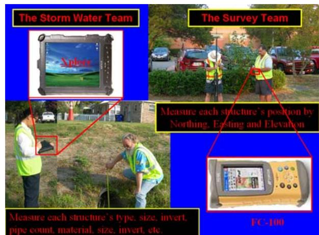
Figure 14. Field Test and Evaluation
