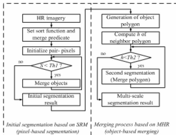
Figure 1. The flowchart of the Multi-scale segmentation based on SRM and MHR.
