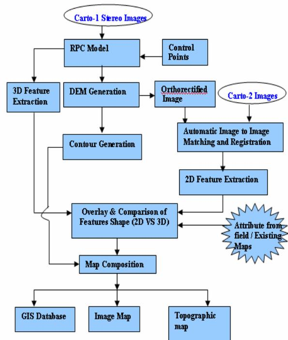
Figure 1: Mapping schematic work-flow frame work
