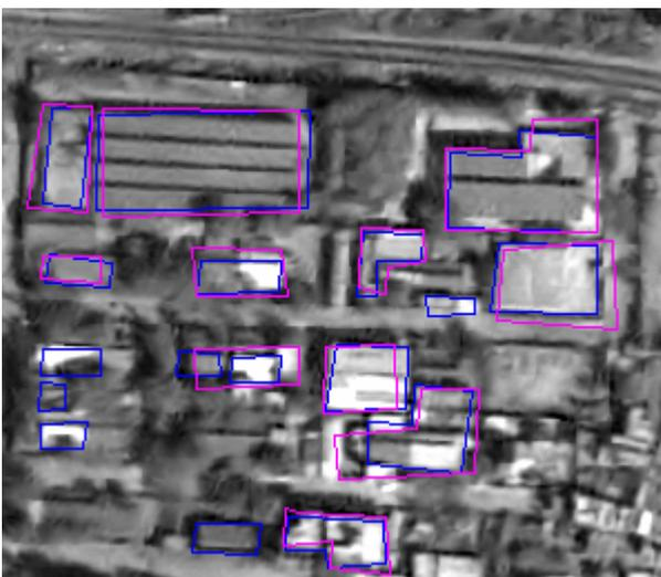
Figure-3 (b) Overlay of features extracted in 2D mode from Cartosat-2 and 3D mode from Cartosat-1 (Magenta: Cartosat-1 & Blue: Cartosat-2) over Cartosat-2 Ortho-image
