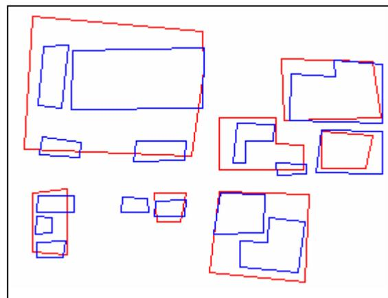
Figure-2(a) Comparison of features extracted in 2D mode (Red: Cartosat-1 & Blue: Cartosat-2)
