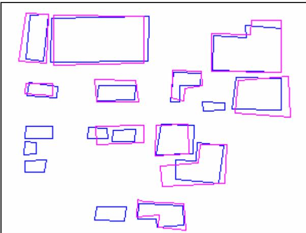
Figure-3(a) Comparison of features extracted in 2D mode from Cartosat-2 and 3D mode from Cartosat-1 (Magenta: Cartosat-1 & Blue: Cartosat-2)
