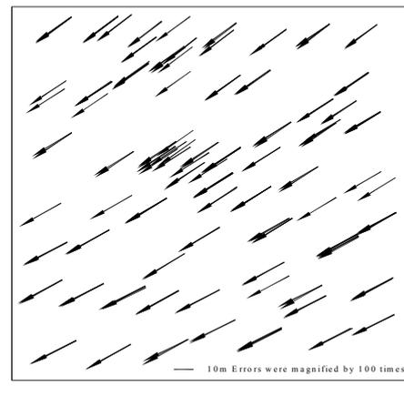
Figure 4. Vector graphics of discrepancies between the RPC generated and GCP coordinates in horizontal direction. The errors were exaggerated 100 times.
