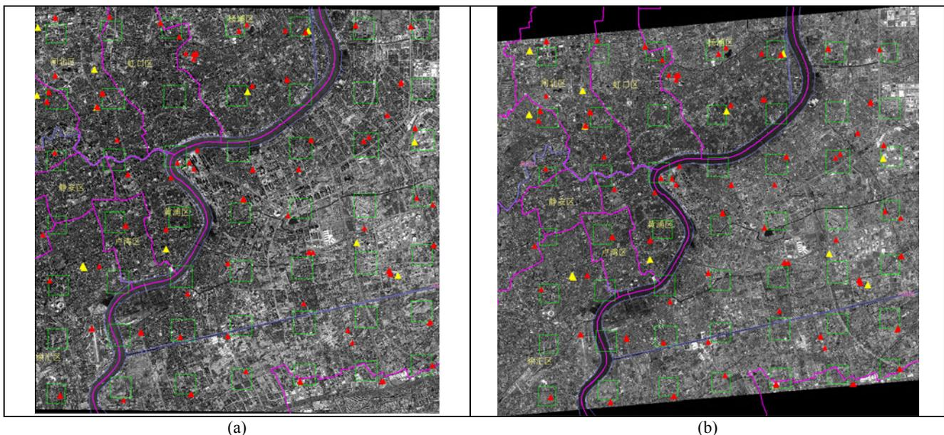
Figure 2. The QuickBird across-track stereo imagery and the distribution of GPS survey points. (a) left (Feb) image of the stereo pair. (b) right (May) image of the stereo pair. The red triangles represent the ground GPS survey points, the yellows ones the building roof survey points. The green rectangles are the 49 districts designed for selection of GPS survey points.
