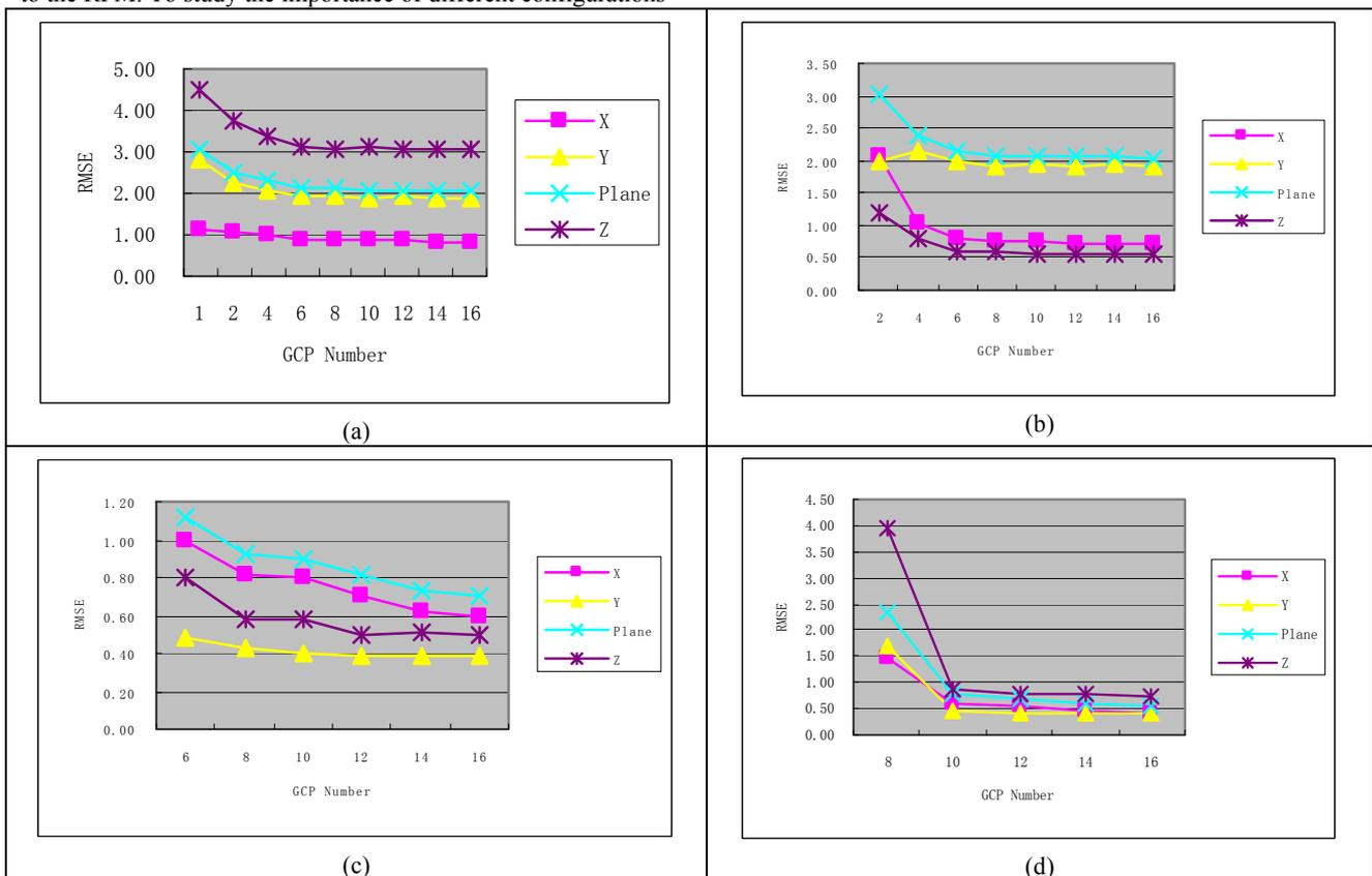
Figure 5. Figures of Accuracy with different GCP Number in object space: (a) .translation model; (b) scale and translation model; (c) affine model; (d) second-order affine model.
