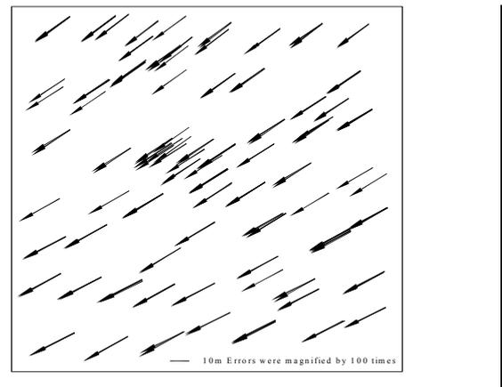
Figure 4. Vector graphics of discrepancies between the RPC generated and GCP coordinates in horizontal direction. The errors were exaggerated 100 times.
