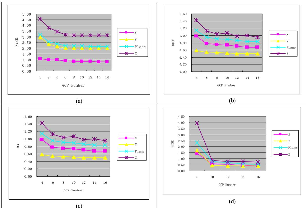
Figure 6. Figures of Accuracy with different GCP Number in image space:
