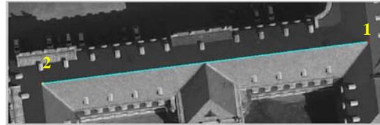
Figure 10. Straight line extracted by the Hough transform
