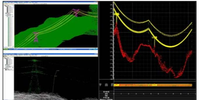
Figure 8. dangerous points checking
