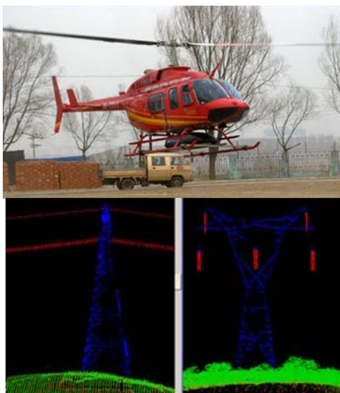
Figure 6. LiDAR system on a helicopter
