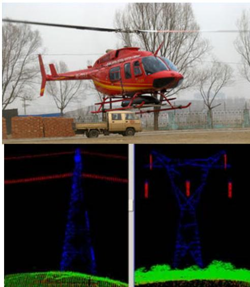
Figure 6. LiDAR system on a helicopter Figure 7. laser points of the tower
