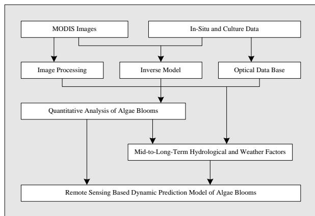
Figure 1. Framework of the model of dynamic prediction model of algae blooms
