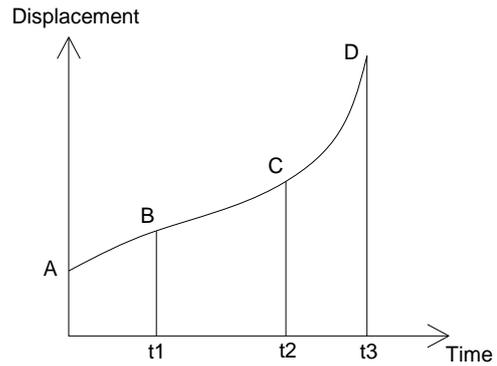
Figure 5. Typical landslide displacement-time curve
