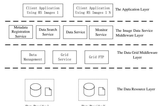
Figure 1. The RS Image Data Sharing Model
