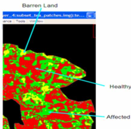
Figure 5. LISS III Images showing the healthy and affected patches obtained from texture based analysis.
