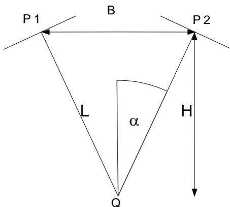
Here: P1, P2 – images, H – altitude, B – photographic base, L – distance from image to ground point, α – angle between vertical direction and line L.
