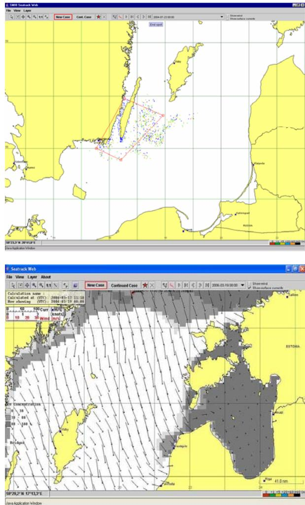
Figure 3. An example of Graphical User Interface for HUMBOLDT Scenario covering Ocean geodata for oil spills monitoring, integrated with SMHI Seatrack Web service. Data from various sources are collected and processed to map the oil spill depth forecasting (upper image) and to foresee the future position of the oil, through the integration of sea current data (lower image).
