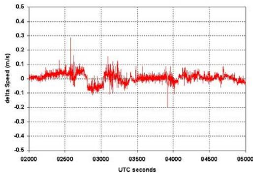
Figure 4. GPS velocity differences between code and RTK solution
