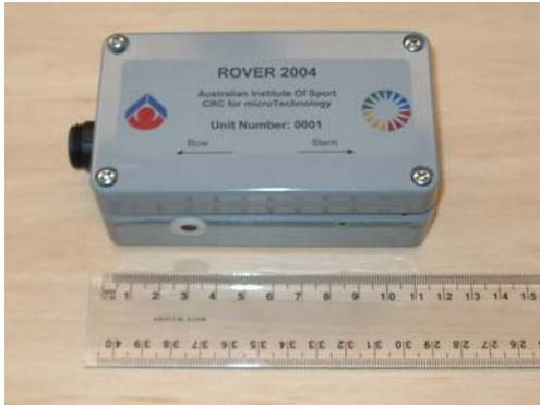
Figure 7. A compact prototype rower monitoring and coaching system (ROVER-2004) with 10 Hz carrier GPS capability and wireless communication.
