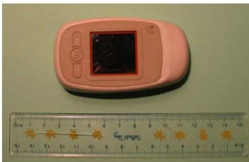
Figure 8. A compact prototype athlete monitoring and coaching system (minimaxX) with high update rate carrier phase GPS capability and wireless communication
