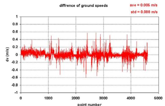
Figure 6. Velocity differences between 10 Hz low-cost GPS and RTK GPS solutions
