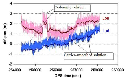
Figure 5. Position differences between 10 Hz low-cost GPS (code-only and carrier-smoothed solutions) and RTK GPS solutions
