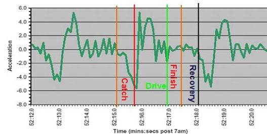
Figure 3. Schematic rowing stroke signature captured from high precision GPS measurements
