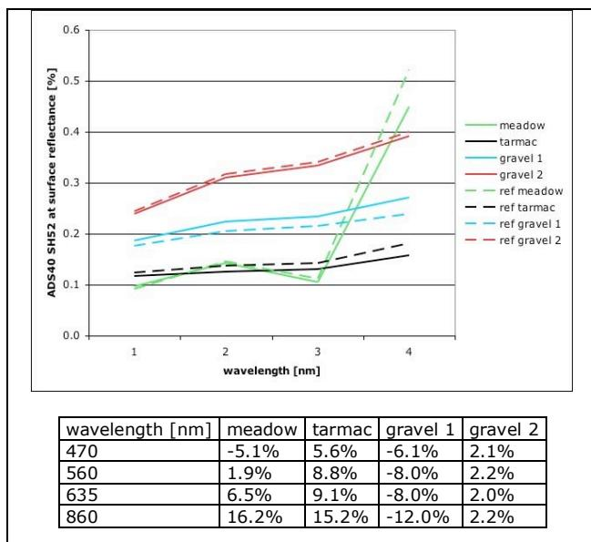
Figure 5. Comparison of ADS40 and ASD-spectrometer at surface reflectance of reference targets, ADS40 sensor head SH40, July 2007, empirical line corrected with ASD targets ,armac’, ,gravel 1’ and ,gravel 2’ of September 2007
