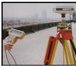
Leica 530 GPS Diplex Signal Receiver (Picture 2)
