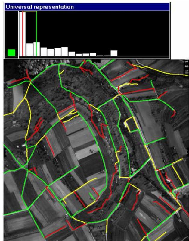
Figure 4. Overview of self-diagnosis. Top: Length-weighted histogram of evaluation scores (left-most bar indicates mean value = green in this example), thin vertical lines indicate thresholds between categories. Bottom: Overview window
