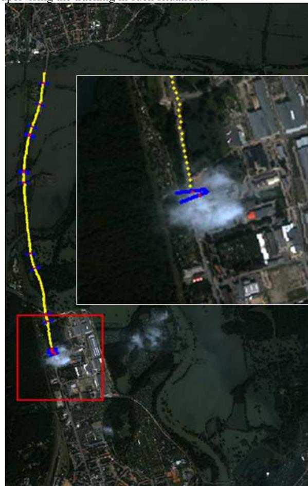
Figure 6. User-assisted road tracking in an IKONOS image taken during the Elbe flooding in Germany, 2002. Yellow: tracked road sections; blue: user clicks.
