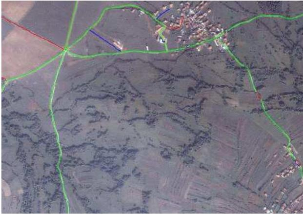
Figure 3. Road extraction from optical satellite image (IKONOS pansharpener). Green: correct extraction; red: missing extraction; blue: false alarms. For more details, see (Mayer et al. 2006)
