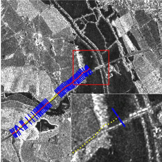
Figure 7. User-assisted road tracking in a RADARSAT SAR image. Yellow: tracked road sections; blue: user clicks.
