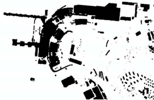
Figure 8. Lidar DSM points located on buildings, extracted using DTM-AV voids and NDVI.
