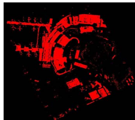
Figure 6. Building class (in red) extracted from intersection of nDSM and NDVI.
