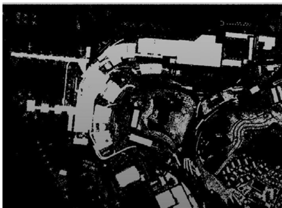
Figure 4. DTM-AV raw data of Zurich airport. The white areas represent voids (buildings, aircrafts, vehicles, high or dense trees).
