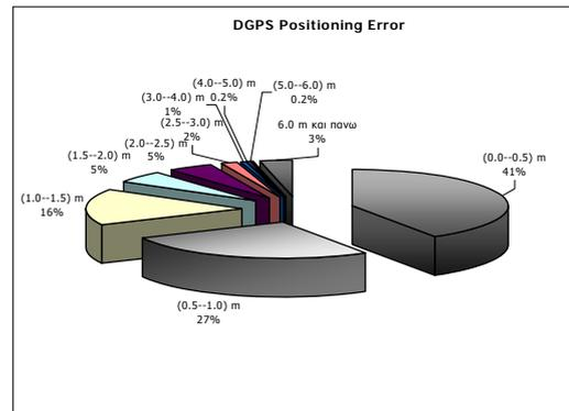
Figure 4. Accuracies of the DGPS solution. In 68% of the cases the accuracy is better that 1 m.
