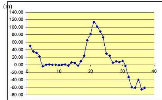
Figure 9. The range of the correction values of the boundaries positions of the parcels
