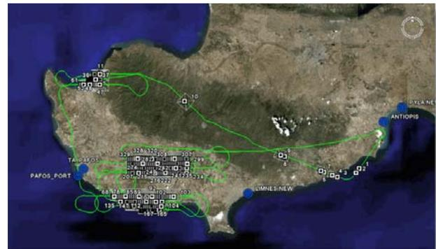
Figure 10. Determination of flight trajectory for direct georeferencing of aerial photography
