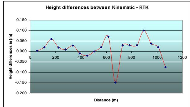
Figure 3. Height differences between Kinematic and RTK solutions
