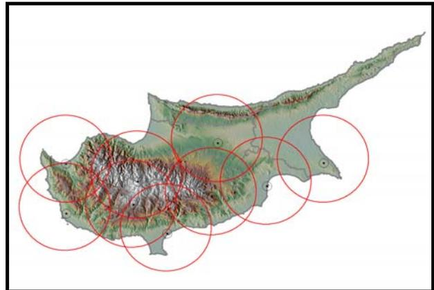
Figure 1. The designed Cyprus permanent GPS network
