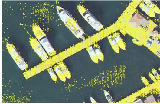
Figure 4. Problems with wharfs or undep water: many points are classified as terrain
