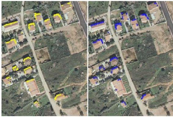
Figure 2. GRASS and TopScan terrain points in the buildings mask. The error is close to the building edge and so it is probably due to the mask itself.
