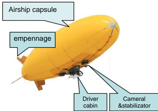
Figure 1. Picture of airship
