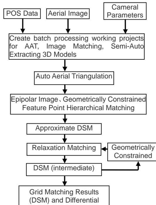
Figure 3. Work flow of building change detection
