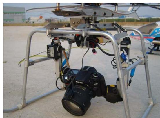
Figure 3. Construction of gimbal mount
