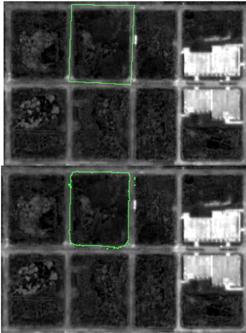
Figure 4. Extract edge of a block. Upper: image with initial curve. Underside: result curve
