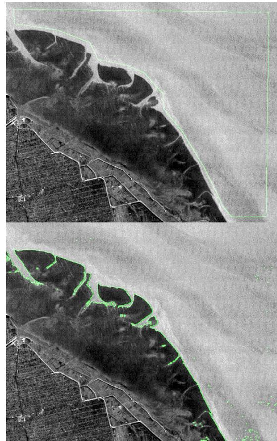
Figure 3. Extract waterline. Upper: image with initial curve.
