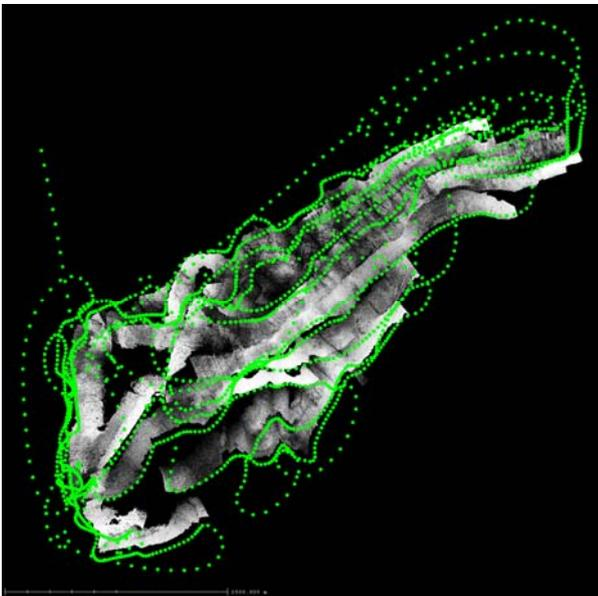
Figure 3. Plot of GPS flight trajectory for Wordiekammen, superimposed over laser point cloud.
