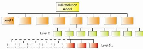
Figure 4. Schematic of octree structure.
