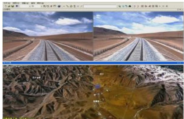
Figure 10. the visualization result of Qinghai-Tibet Railway, China (the total length of Qinghai-Tibet of 2284km, data collection spends 7 days, data processing spends 10 days, resources include 2 operators, 1 MMS vehicle and 1 railcar)
