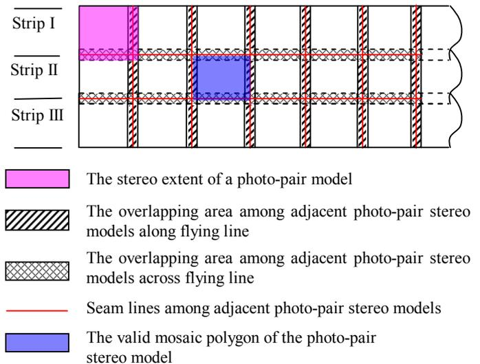
Figure 3. The arrangements of photo-pair models
