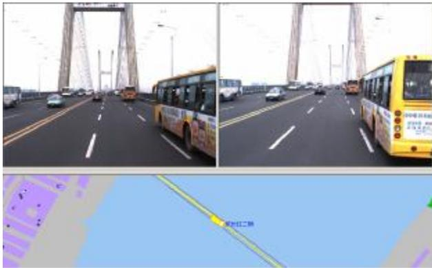
Figure 12. the Integration result of DMI and electric map in vector format
