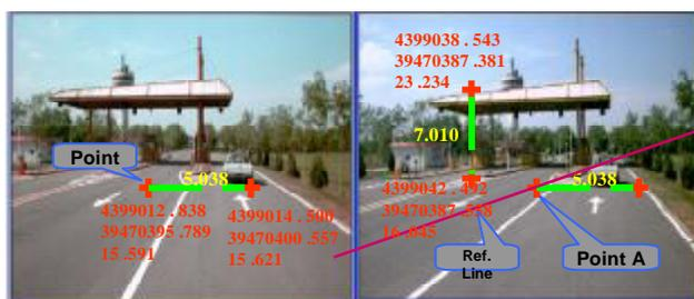
Figure 13. Measurement of road width and object height by end users on web
