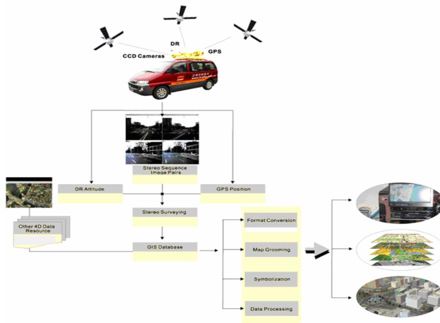
Figure 6. The working principle of VisionCruiser™
