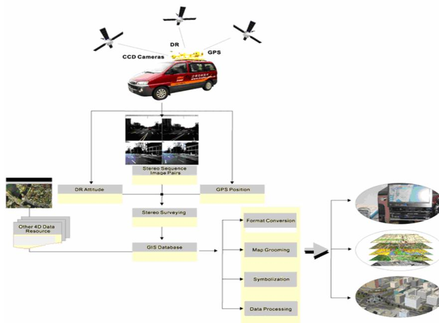
Figure 6. The working principle of VisionCruiser™
