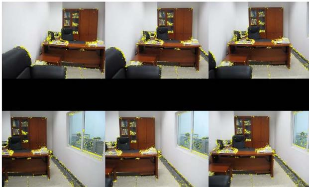
Figure 2. Feature points detected by SIFT algorithm. Six images from a sequence of indoor scene. The image size is 800\*600 pixels, and about 1000 features are detected in each image. Because of redundant keypoints at different scales there will be several duplicate points around a keypoint when transferred to original images. However feature point descriptors at multi-scales makes matching result invariant to scales.
