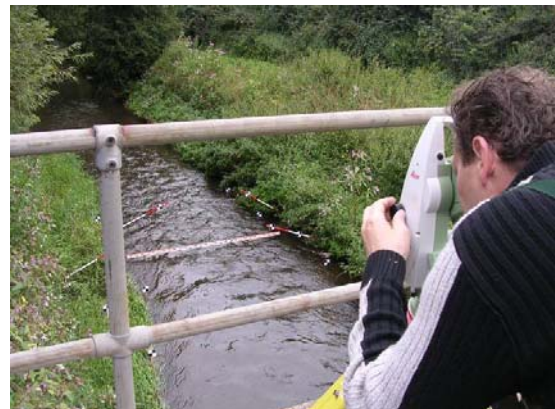
Figure 4 Experimental setup to measure a dynamic water surface on a small river at Loughborough
