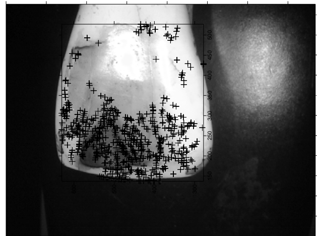
Figure 3. Distribution of 600 successful matches on a limited region of the tooth, shown superimposed on the monochrome left image. The paucity of points in the vicinity of glare and light texture is very apparent.
