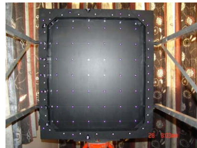
Figure 1. A convergent image used in the system calibration. Note the temporary retro targets (inside the control frame) used for lens distortion calibration.
