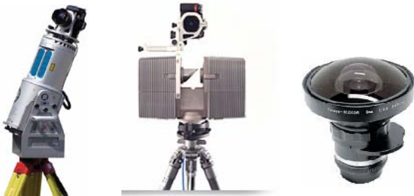
Figure 1. Laser scanner and camera: Riegl LMS-Z420i with Nikon D100 (Riegl, 2007); FARO LS 880 with Nikon D200 and Fisheye lens (Faro, 2005); Nikkor Fisheye lens 8 mm
